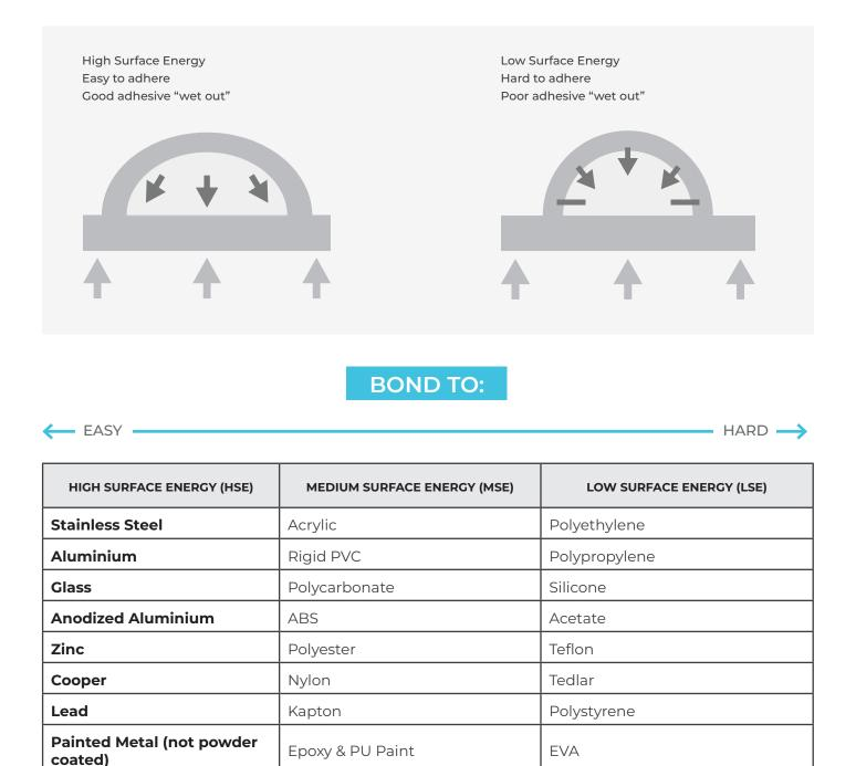
NOTE: The higher the surface energy, the greater the strength of adhesion.
